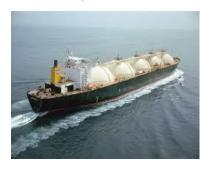
Liquefied Natural Gas is natural gas that has been super-chilled to -260 degrees, turning it into a liquid that is 1/600th the original volume of gas. It is clear, colorless, odorless, and extremely volatile. This gas is compacted so large volumes can be shipped overseas. LNG should not be confused with gasoline or compressed natural gas.
