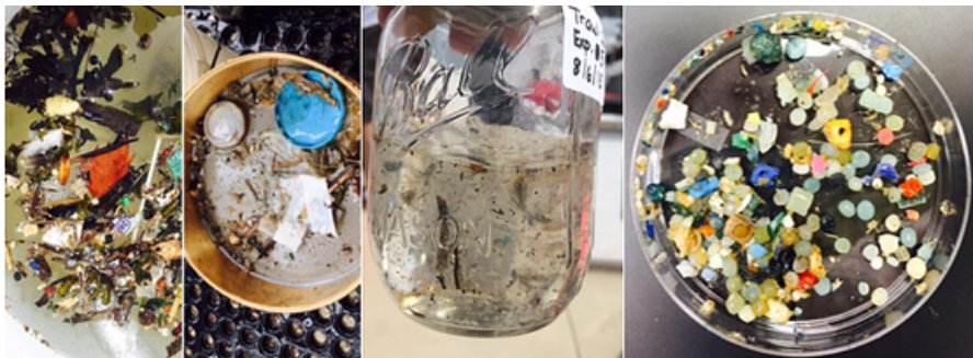
(LEFT TO RIGHT) Contents of a trawl, contents being sieved, a preserved sample before lab processing, and microplastics after lab processing prior to categorizing and counting.
