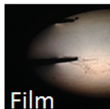
(BELOW left-to-right) An image of the five types of microplastic particles: 1) fragment- hard jagged piece of plastic, 2) pellet- round hard particles of plastic, 3) film- clear/white flimsy planes of plastic, 4) fiber- clear/colored lines of plastic, and 5) foam- sponge-like pieces of plastic
