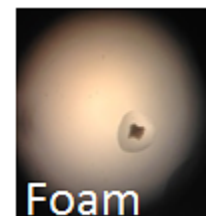
(BELOW left-to-right) An image of the five types of microplastic particles: 1) fragment- hard jagged piece of plastic, 2) pellet- round hard particles of plastic, 3) film- clear/white flimsy planes of plastic, 4) fiber- clear/colored lines of plastic, and 5) foam- sponge-like pieces of plastic
