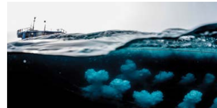
A ship operates an air-gun array while looking for oil deposits off the coast of Greenland. Photo: https://www.nature.com/news/air-guns-used-in-offshore-oil-exploration-can-kill-tiny-marine-life-1.22167 courtesy of Christian Aslund / Greenpeace
